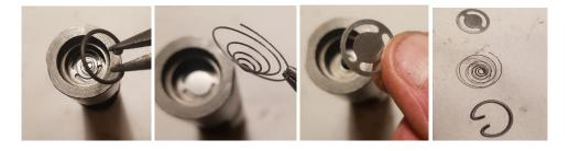
13. Assembly the valve with the center top of the spring facing down against the aluminum disk. See that the "lose end" on the big diameter of the spring is not hooking in to or getting caught in the grove for the circlip when the circlip is put back.
