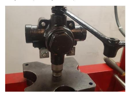
30. Align and press the other *damper arm* onto the axle on the other side. Make sure that the *damper arms* are mowing freely. There will be som resistance because of the (old fashion) *rubber seals*.
