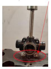
8. Press out the *axle shaft*. See that the *damper arm* under is not hooked up in anything while pressing the *axle* and *damper arm* down.
