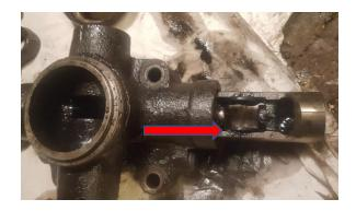
12. Be careful with the two valves with small circular conical springs at each end of the *piston*. They are the *recuperating valves* that let the oil flow through to the front of the *piston* when the *piston* is moving from side to side. (Returning after a compression stroke.) They can be removed by taken out the circlip and carefully take of the conical spring. Remove the aluminum disk and clean the disk and its seat.
