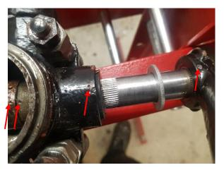
7. Arrange it so the *damper housing* can rest steady on its side in the hydraulic press, with the *splined damper arm* facing down through a hole in the footboard /base plate. (See photo)
